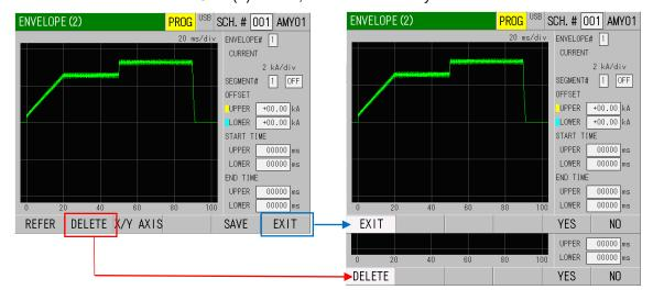
7) Touch the REFER key to take in the reference waveform. The waveform measured in 3) is displayed. Based on this waveform, set the time range for upper and lower limits.
