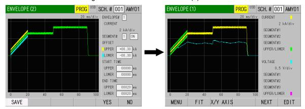
11) Touch the EDIT key again, select 2 for SEGMENT#, and change OFF to ON. Perform steps 6) to 10). Be sure to perform from REFERENCE to SAVE for each setting of SEGMENT.
