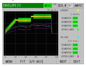
② How to create the upper/lower limit threshold based on the optionally created waveform
