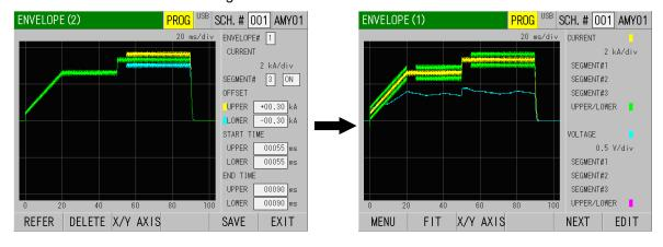
13) Similarly, select 2 for ENVELOPE# for WAVEFORM 2 and perform settings of SEGMENT#1 to 3. Be sure to perform from REFERENCE to SAVE for each setting of SEGMENT.
