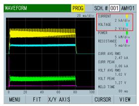
3) Insert the USB into the **MM-400B** and select WAVEFORM for ITEM in the USB screen. Set the interval to sample from waveform data in WAVE DECIMATION, and then touch the SAVE key. "¥wav" folder is created in the USB and the waveform's CSV file (any of "wav-0.csv" to "wav-1000.csv") is created in the folder. Confirm that sampled interval time is input in column A and WAVEFORM 1 to 4 data of each sampled interval are input in columns B to E. Item names of waveform in the CSV are as follows.
