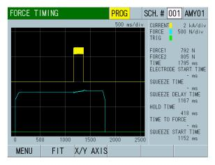
Way to start measurement using the external input signal "FORCE TRIGGER" (force valve driving signal) together
