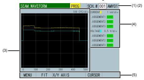
Waveform of intermittent seam current / voltage
