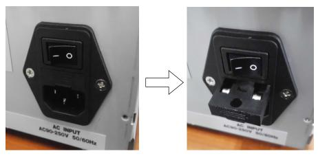
2) Remove the broken fuse.
