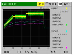
14) The envelope setting is complete. Make measurements on the ENVELOPE (1) screen and check the setting contents by waveforms.
