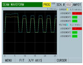
The **MM-400B** realizes seam welding by repeating measurement of the specified range. The measured value calculated with the measurement range and the measurement interval is displayed.
