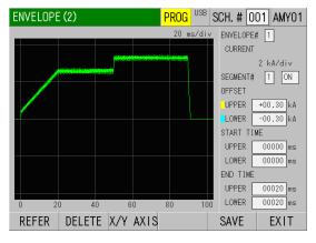
9) Touching the REFER key and selecting YES displays reference waveform and envelope setting. You can also check the detailed data of time axis and vertical axis by touching the X/Y AXIS key. After check, touch the BACK key and return till the REFER key is shown.
