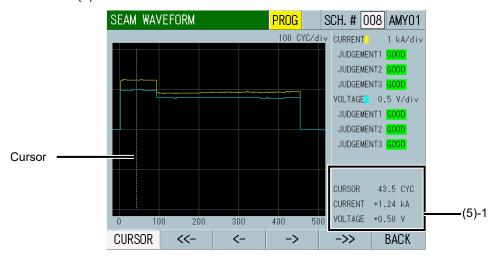
Shows the current time axis information of the cursor and the measured values of the waveforms at the point in time indicated by the cursor.
