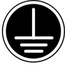
Connect the grounding cable to the grounding terminal located near the grounding mark.
