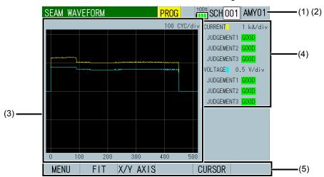
Waveform of intermittent seam current / voltage
