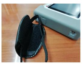
3) Fix the belt to the hook and loop fastener of the cushion.
