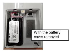
4) Hold the connector and pull it upward to remove the battery.
