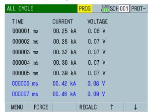
Left: Measured value before recalculation Right: After recalculation
