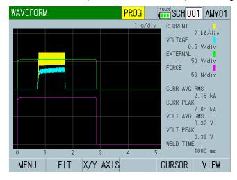
Displays ON (+0 V) to 500 N (+10 V) with a load cell amplifier prepared separately.
