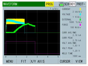
Displays  $140^{\circ}$ C (4 mA) to  $2000^{\circ}$ C (20 mA) with a radiation thermometer. Less than  $140^{\circ}$ C is not displayed.
