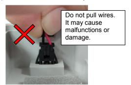
5) Connect the connector of the replacement battery to the connector of the instrument, and then house the battery body in the box.
