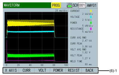
X AXIS: Touching this enlarges/reduces the time axis of waveform and makes it possible to move the waveforms. In this condition, touch the arrow key (<- ->). This moves the waveforms to the right or left. Touch + (plus) to enlarge the time axis of waveform or - (minus) to reduce it.
