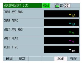
To display a waveform or change or check the setting, touch MEAS to change it to PROG. (Alternately switched by touching.)
