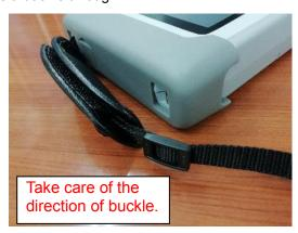
6) Pass the belt through the pin at the lower part on the left side of the **MM-410B**.
