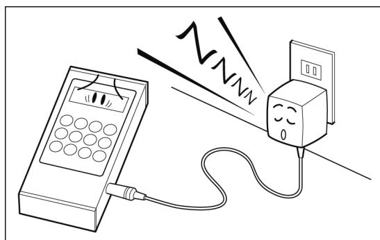
■ Do not short-circuit the plug while the charger is connected to an outlet.
