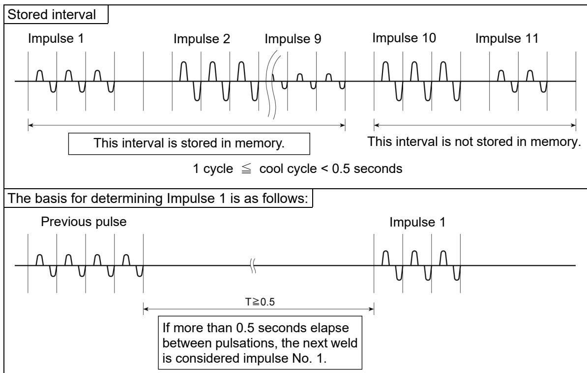
All previous memory information is cleared when the power is shut off or a new weld is performed.
