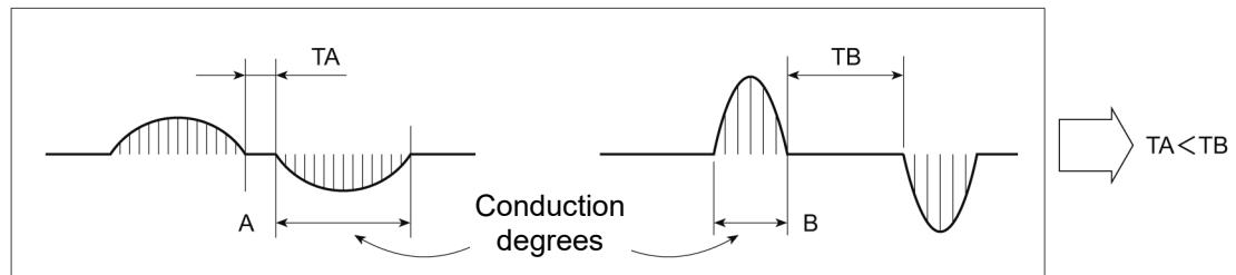
Though the RMS current values are the same, the time during which the current doesn't flow differs (TA in A, TB in B).
