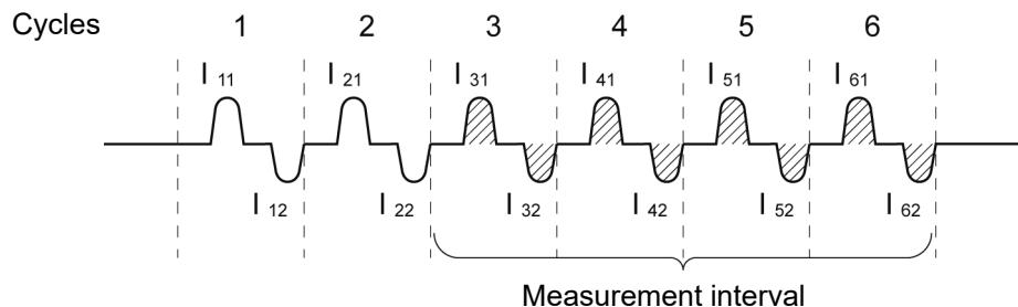
$$\text{Displayed current} = \frac{\text{Average true values}}{8} = \frac{I_{31} + I_{32} + I_{41} + I_{42} + I_{51} + I_{52} + I_{61} + I_{62}}{8}$$
