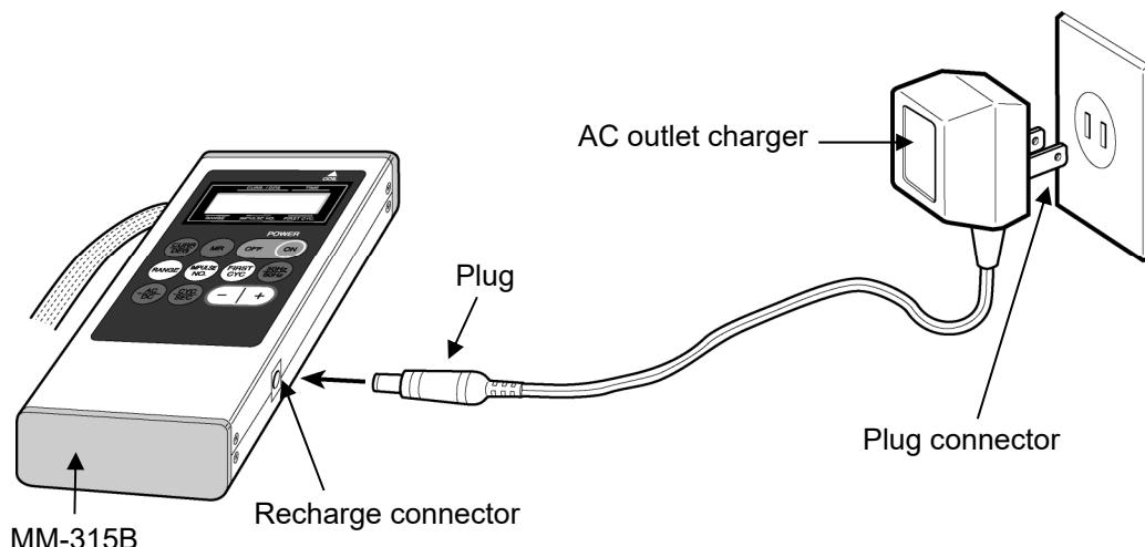
Connect the plug to the recharge connector of the unit, and plug the charger into an outlet. Fifteen hours are required to fully recharge the unit. Do NOT charge for more than 48 hours. Excessive charging will shorten the service life of the batteries. Be sure to charge at a room temperature of 35°C or lower.
