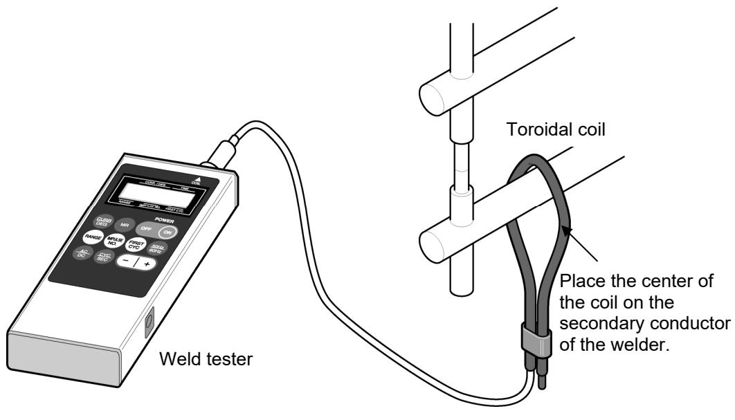
Line up the ends of the coil, and fasten both ends using the Velcro strips.
