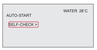
The laser checks the opening/closing status of branch shutters, memory (sum check and data range), and charge trouble automatically. If no trouble is found, the KEY-SWITCH ON > screen appears.
