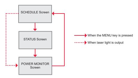
When the power supply is turned ON with the CONTROL keyswitch OFF and the MENU key pressed.
