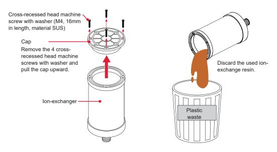
⇒ Dispose of the used ion-exchange resin together as plastic waste.
