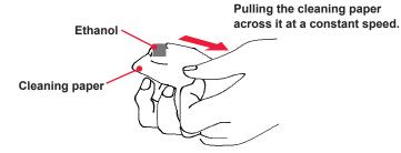
⇒ If any clearance is produced between the cleaning paper and the optical part or ethanol is left during wiping, this will result in unevenness.
