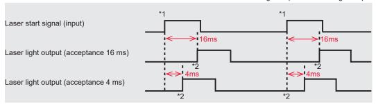
⇒ The laser start signal acceptance time and the schedule signal acceptance time are common. A different value cannot be set for the respective time.
