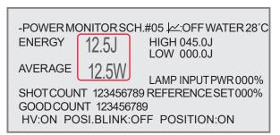
Move the cursor to "" and press the ON key. Then, the numeric values of laser output are graphically displayed and you can check them by waveform.
