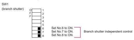
The independent control of the branch shutter is set and the items "MIRR-1" and "MIRR-2" to operate the timesharing unit are displayed on the STATUS screen. Laser light can be output according to an optional specification resulting from combining "BEAM-1", "BEAM-2", "BEAM-3", "MIRR-1", and "MIRR-2."
