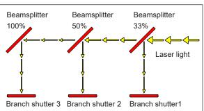
Laser light is reflected on the beamsplitter and split, and then simultaneously transferred from opened branch shutters 1, 2, and 3.
