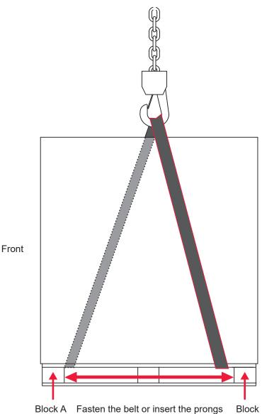
Block A Fasten the belt or insert the prongs Block B of the lift truck between these blocks.
