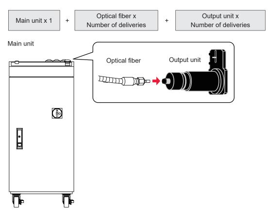
The ML-2050A/2051A/2150A main unit is provided with the number of branch shutters with open-close sensor based on the number of deliveries.
