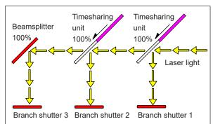
Laser light is reflected on the beamsplitter by operated timesharing unit and transferred from opened branch shutter 3.
