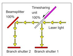
Laser light is reflected on the beamsplitter by operated timesharing unit and transferred from opened branch shutter 2.
