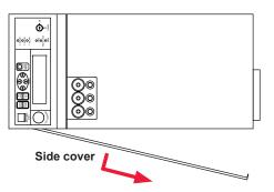
Loosen the screw at the rear of the cover and pull it forward, and then pull it obliquely backward.
