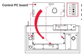
**Right Connector** Insert the two pins on the PC board underneath into Pins 3 and 4 on the control PC board.
