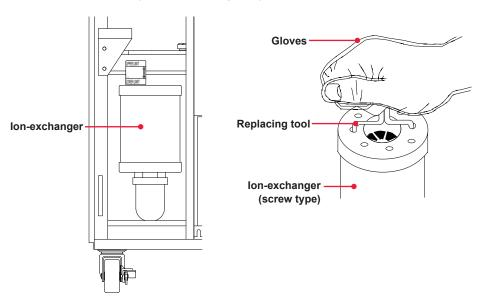
(4) Remove the cap of the ion-exchanger and discard the used ion-exchange resin.
