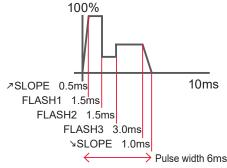
⇒ At the leading edge of waveform, an overshoot (higher form than the set value) may occur. In this case, extend "¬SLOPE" by 0.1 to 1.0 ms.
