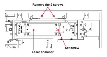
(4) Remove the 2 screws and then remove the lead wire of the flashlamp. Remove the 4 bolts and then remove the upper chamber. Put it upside down on a clean cloth so that its inside may be visible.
