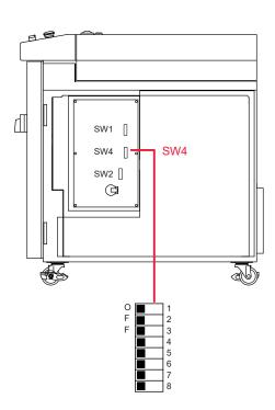
The 4 types of acceptance time of 1 ms, 4 ms, 8 ms, and 16 ms are available. At delivery, the acceptance time is set to 16 ms. To change this setting, switch the ON/ OFF status of No.1 and No.2 of SW4 as shown below.
