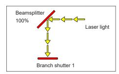
Laser light is reflected on the beamsplitter and transferred from opened branch shutter 1.
