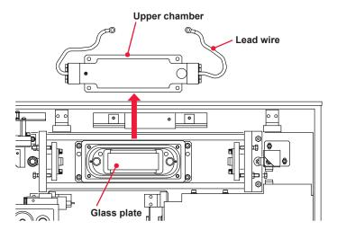
The laser chamber consists of an upper part and a lower part. In the lower chamber, the glass plate is put on the reflector.
