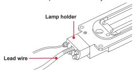
(2) Slowly pull out the flashlamp from either side. At this time, straighten the lead wires so that their terminals will not scratch the reflector panel.
