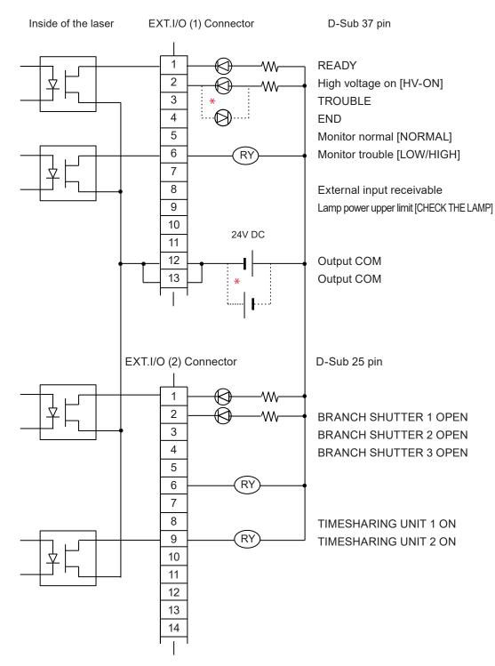
Type of output: Photo MOS relay output Rating of output: 24 V DC, 20 mA max.
