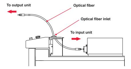
(4) Connect the fiber to the laser beam input unit, with the key of the fiber plug aligned with the groove of the unit.
