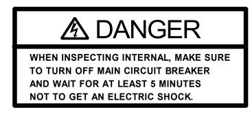
Location: Power Supply interior, side surface of acrylic cover. Meaning: **Danger.**
