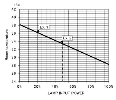
The chart at left depicts the cooling capability at 100% duty cycle. Do not use in room temperature exceeding the line shown.
