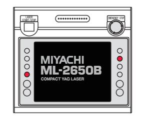
(2) While the model name screen is displayed (for about 3 seconds), press the right and left buttons (red portions in the above figure) of the laser controller simultaneously for 2 seconds.
