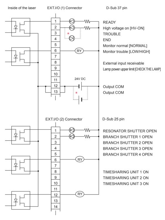
Type of output: Photo MOS relay output Rating of output: 24 V DC, 20 mA max. \* The polarity may be positive or negative. Maintenance Part Appendixes
