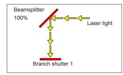
Laser light is reflected on the beamsplitter and transferred from opened branch shutter 1. The timesharing unit is not installed.
