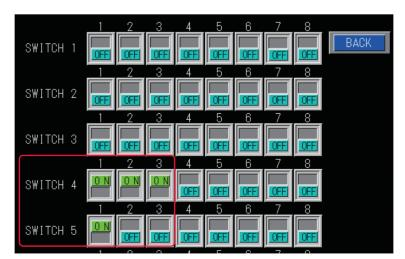
In the case of 2-powersharing delivery + single delivery, laser light is output from branch shutters 1 and 2 as 2-powersharing delivery and from branch shutter 3 as single delivery, depending on a difference in beamsplitter mounting condition.
