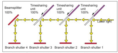
Laser light is reflected on the beamsplitter by operated timesharing unit and transferred from opened branch shutter 1 to 4.
