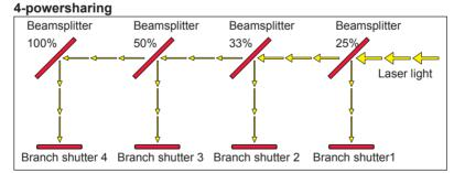
Laser light is reflected on the beamsplitter and split, and then simultaneously transferred from opened branch shutters 1, 2, 3, and 4.
