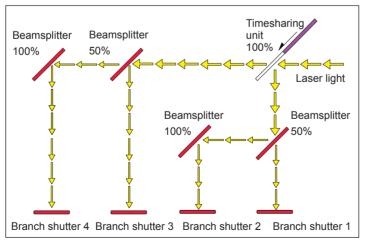
Laser light is reflected and branched on the front or rear beamsplitter by the operation of the timesharing unit. The beams are simultaneously transmitted when branch shutters 1 and 2 or 3 and 4 are opened.
