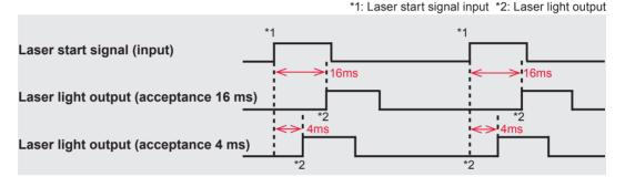
⇒ The laser start signal acceptance time and the schedule signal acceptance time are common. A different value cannot be set for the respective time.
