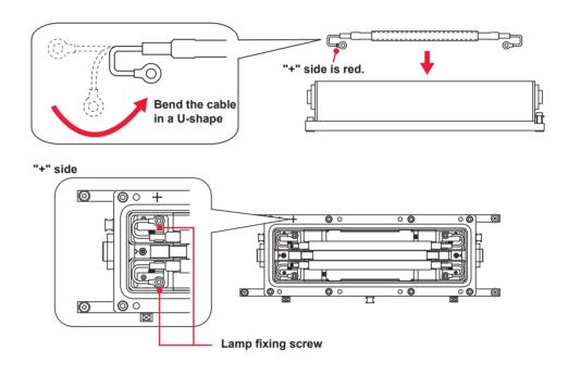
(3) Tighten the bolts on both ends of the flashlamp to fix the flashlamp.<Note>
