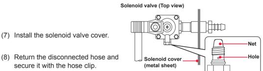
(8) Return the disconnected hose and secure it with the hose clip.
