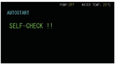
The resonator shutter, timesharing unit, branch shutter, memory, and power supply unit are automatically checked. When no error is found, the KEYSWITCH !! screen is displayed.
