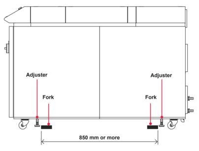
Figures below show example forking; insert the forks fully till the points appear from under the Laser.
