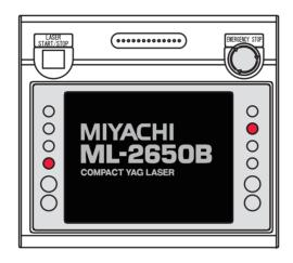
(2) While the model name screen is displayed (for about 3 seconds), press the right and left buttons (red portions in the above figure) of the laser controller simultaneously for 2 seconds. The INITIAL IZE screen appears
