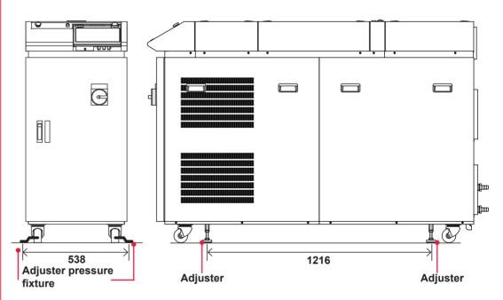
(2) Fix each adjuster on the floor by using a connecting apparatus such as anchor.
