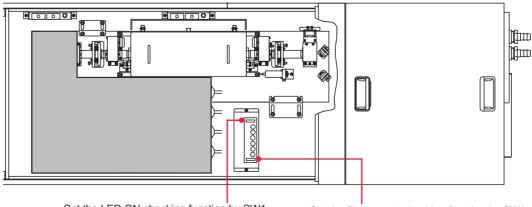
Set the LED ON checking function by SW1.
