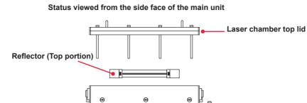
(4) Loosen the bolts of both ends of the flashlamp. Hold both ends of the flowtube (glass tube) with both hands and lift it up together with the flashlamp.
