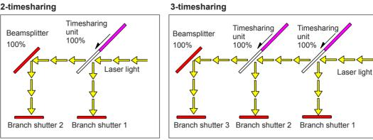
Laser light is reflected on the beamsplitter by operated timesharing unit and transferred from opened branch shutter 2.
