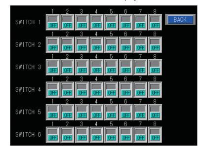
(2) Press the setting buttons of "1" to "4" of "SWITCH 4" to set the branch shutter No. to be operated to ON.
