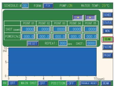
(1) Press the "SEAM" button to display the SEAM screen.
