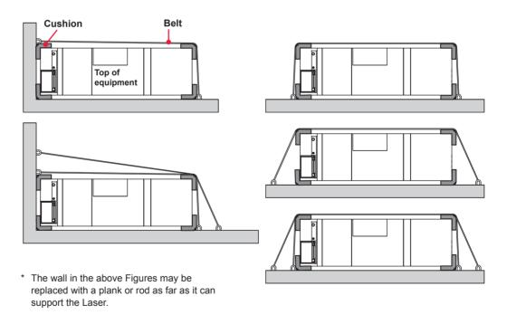
⇒ When it is expected that the Laser may bounce during transportation, belt the Laser longitudinally.
