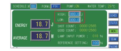
When laser light is out of the set allowable energy range, a monitor error is output.
