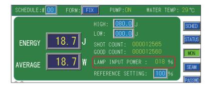
The set ratio of the upper limit value is registered. When the upper limit value is exceeded, a screen to prompt the operator to replace the flashlamp is displayed.
