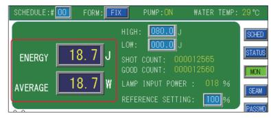
Setting example after switching ("6" of SWITCH 1: ON)
