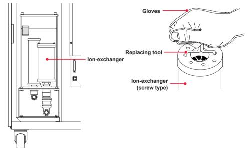
(4) Remove the cap of the ion-exchanger and discard the used ion-exchange resin.
