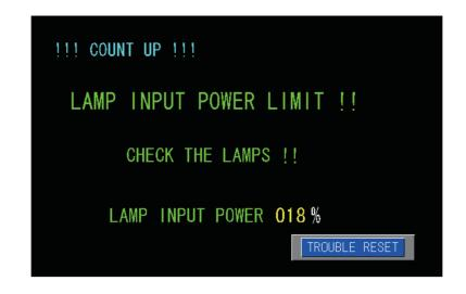
When this screen appears, output pin No.9 (upper limit of lamp input) of the external output signal EXT.I/O (1) connector is open-circuited for output.
