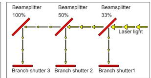
Laser light is reflected on the beamsplitter and split, and then simultaneously transferred from opened branch shutters 1 and 2.
