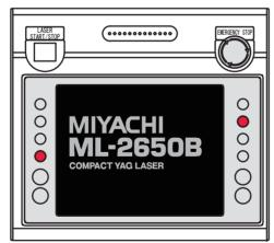
(2) While the model name screen is displayed (for about 3 seconds), press the right and left buttons (red portions in the above figure) of the laser controller simultaneously for 2 seconds.
