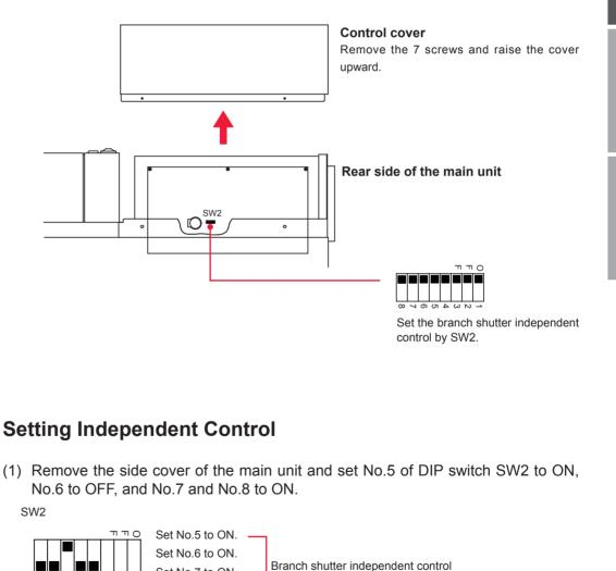
The branch shutter independent control is set and the MEMORY SWITCH screen is displayed from the INITIALIZE screen. As a result, it is possible to set that only an optional branch shutter and timesharing unit can be operated.
