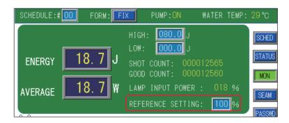
⇒ If the laser welder is used in the status where 80% or more is displayed in "LAMP INPUT POWER", the flashlamp replacement cycle may be shortened.
