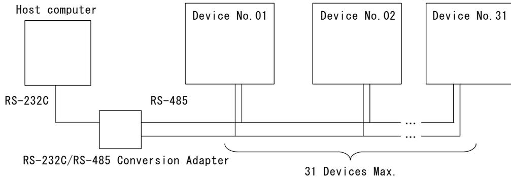
(Note 1) When controlling two or more devices with one host computer, register the device No. (**CONTROL#**) for each device. Set the device No. at POWER SUPPLY STATE screen (See 4.(2)(b)).
