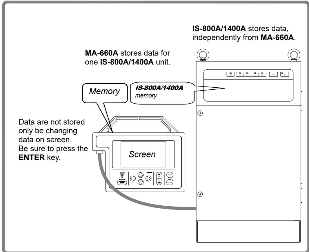
When two or more the Power Supply units are used and the contents of the memory of the first unit need to be copied to the second unit, copy the data from the first unit to the memory of **MA-660A** temporarily, then copy this data to the second unit.
