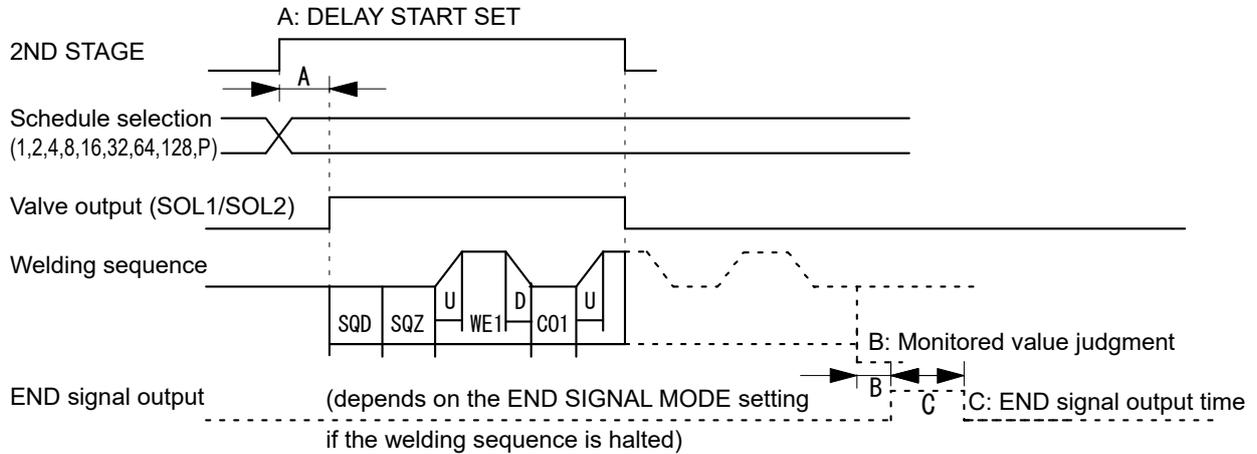
(Note) When OFF/Off time is set, MAINTAINED does not work. It works as LATCHED.
