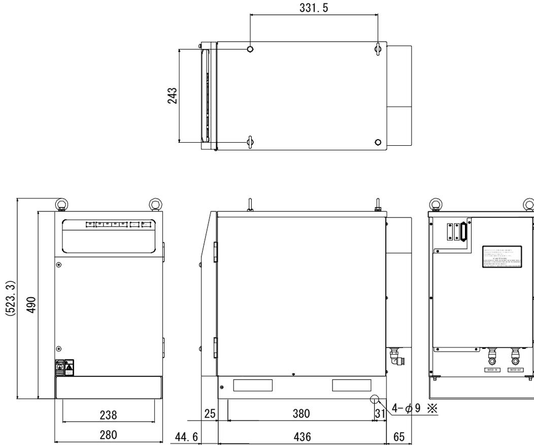
\* For fixing the Power Supply. Remove the cover plate on the base front to tighten screws.
