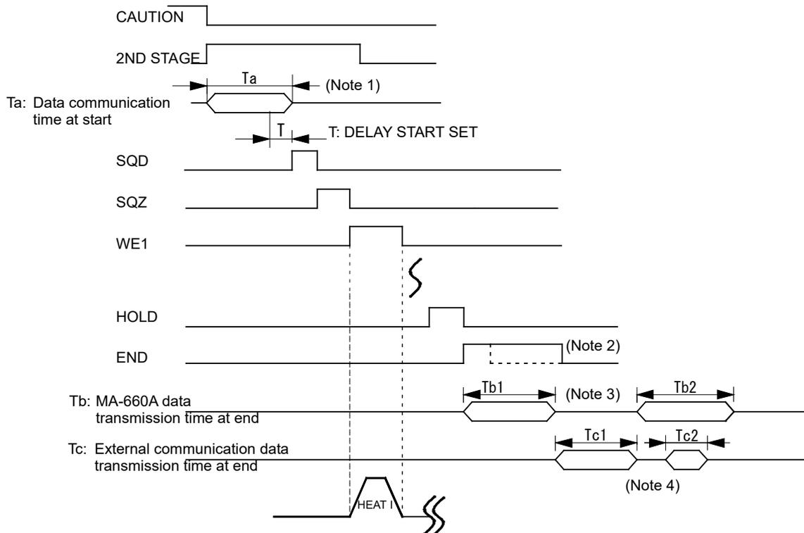
(Note 1) When the next start signal is received while the monitor error is displayed on **MA-660A**, the CAUTION signal is turned OFF and the previous screen is displayed.
