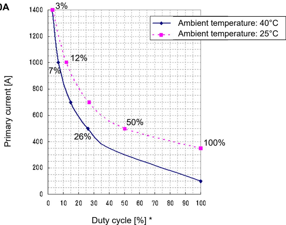
\* This duty cycle graph is applied when the frequency is set to 1 kHz. Decrease the duty cycle by 0.5% (from the above graph) for each additional 100 Hz of frequency. (Example: When the frequency is increased to 3 kHz, the duty cycle needs to be decreased by 10%.)
