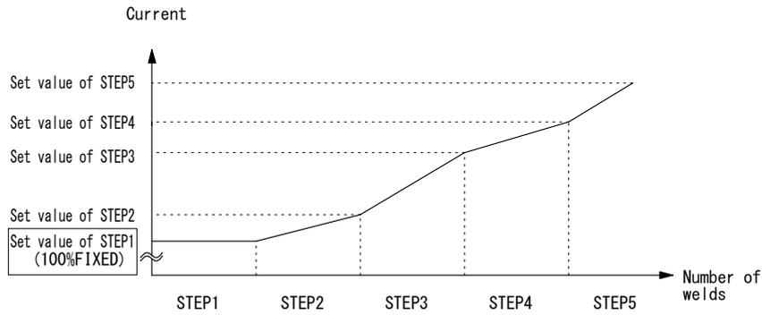
As shown in the above figure, the current is stepped up or down to the value for **STEP2** with the specified number of welds for **STEP2** following completion of the specified number of welds for **STEP1**.
