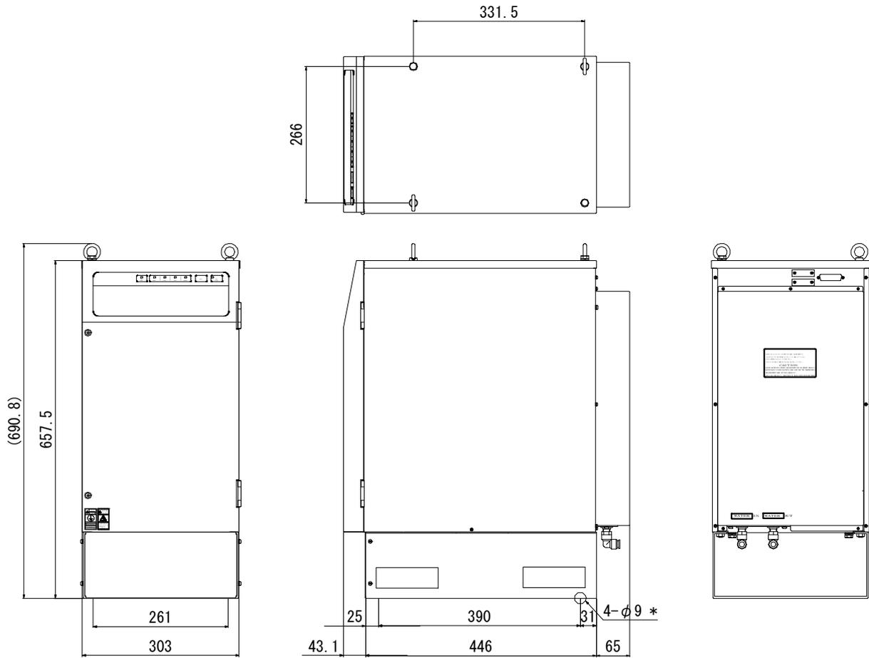
\* For fixing the Power Supply. Remove the cover plate on the base front to tighten screws.
