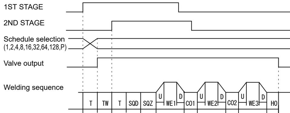
When the 2ND STAGE signal is input, the valve signal with the selected schedule number is output. After the welding sequence starts, the valve signal is output until the sequence ends even if the 2ND STAGE is turned OFF.
