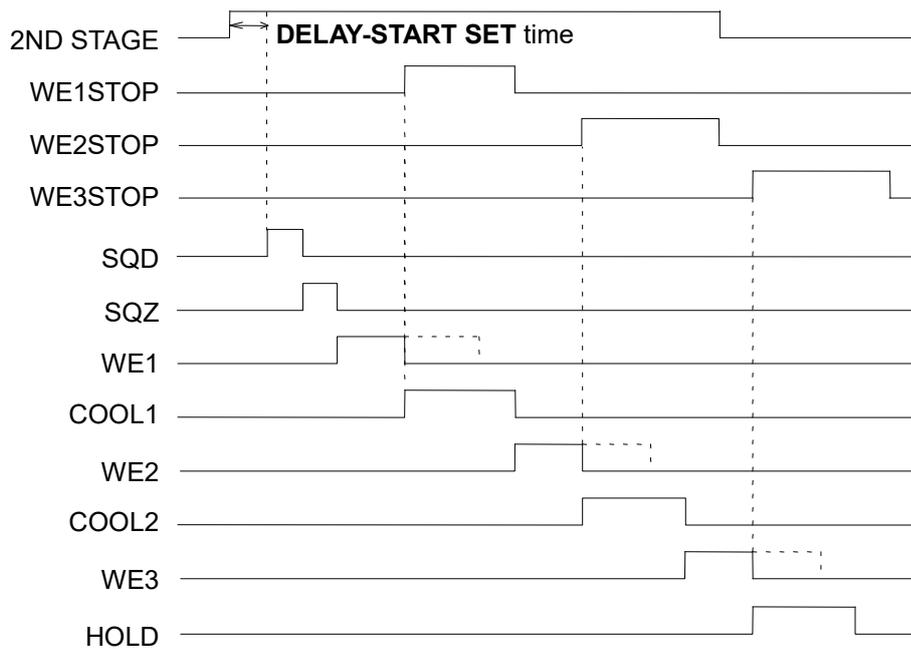
The **WE1 STOP** signal shuts off current immediately when input during the **WE1** period, switching the sequence to **COOL1**. The **WE1 STOP** signal shuts off current immediately after the **WE1** starts (the current is supplied for about 1 cycle) when input before the **WE1** period, switching the sequence to **COOL1**. The **WE1 STOP** signal will not shut off current if input during the **WE2** or **WE3** period.
