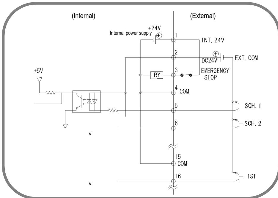
(Note) The circuit between pins 1-2-3, 4-5, 18-19-20, and 21-22 are closed when shipped. Disconnect unnecessary jumper wires referring to each connection.
