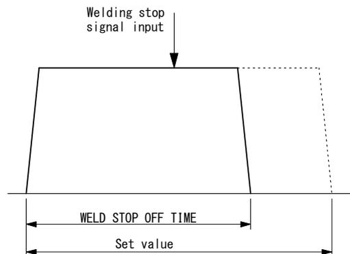
② When the welding stop signal is input after WELD STOP OFF TIME
