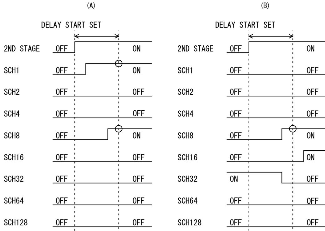
In Fig. (A), schedule signals 1 and 8 are **ON**. Therefore, welding is performed using schedule No. 9. In Fig. (B), only schedule signal 8 is **ON**. As a result, welding is performed using schedule No. 8. Schedule signals 16 and 32 are invalid because they are **OFF** when the schedule is determined.
