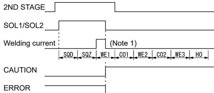
(Note 1) When caution or error occurs, subsequent welding sequence is not performed.
