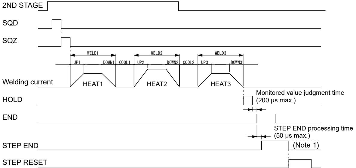
(Note 1) The STEP END output is ON until the STEP RESET signal is received.
