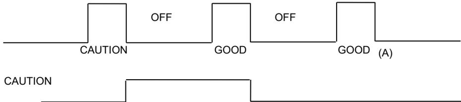
When the sequence is stopped at (A), error (CAUTION) is not displayed. It's because the contents when stopped is displayed on the program unit.
