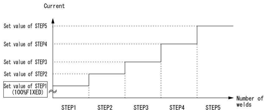
As shown in the above figure, the current is stepped up or down to the value for **STEP2** following completion of the specified number of welds for **STEP1**. Similarly, the current is stepped up or down to the value for **STEP3** following completion of the specified number of welds for **STEP2**.
