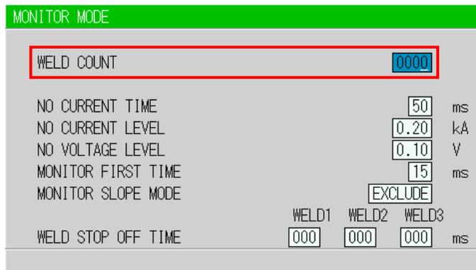
A count error signal is output if the number of welds deposited while the
