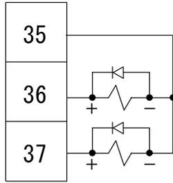
\*3 When solenoid valves are activated by the use of an internal power supply
