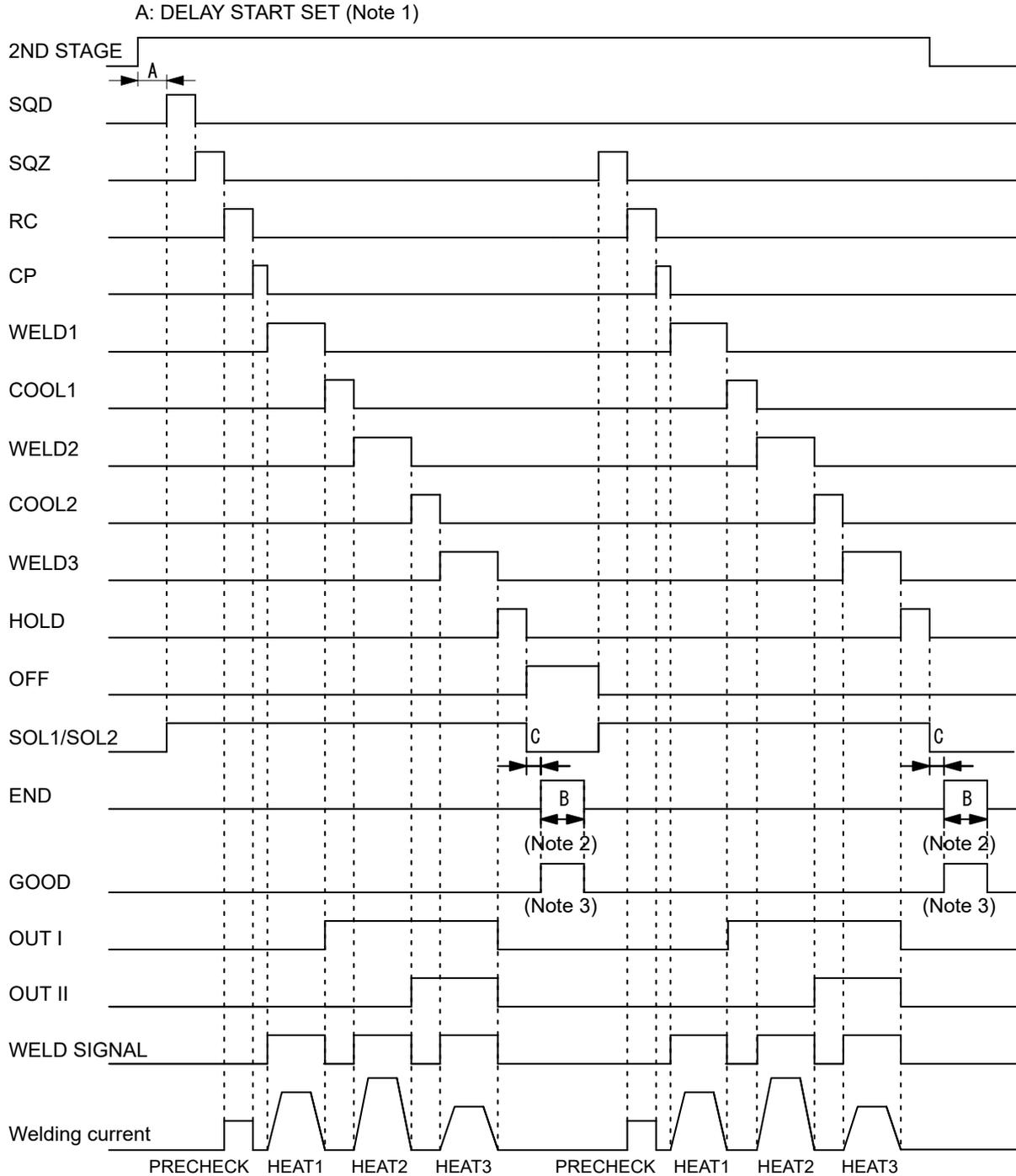
SQD: Squeeze delay time    SQZ: Squeeze time    RC: Resistance precheck time
