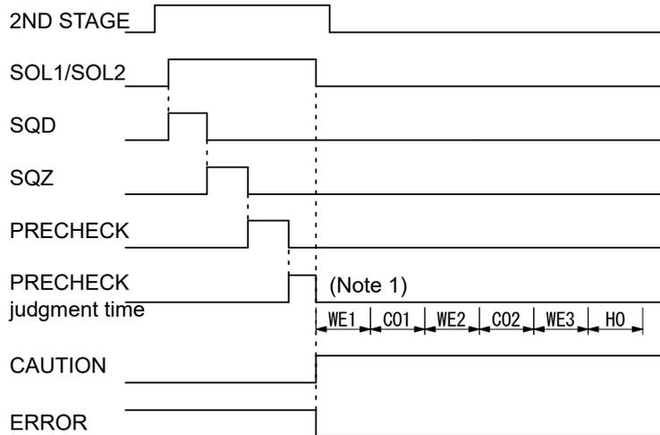
(Note 1) When the precheck caution or error occurs, subsequent welding sequence is not performed.
