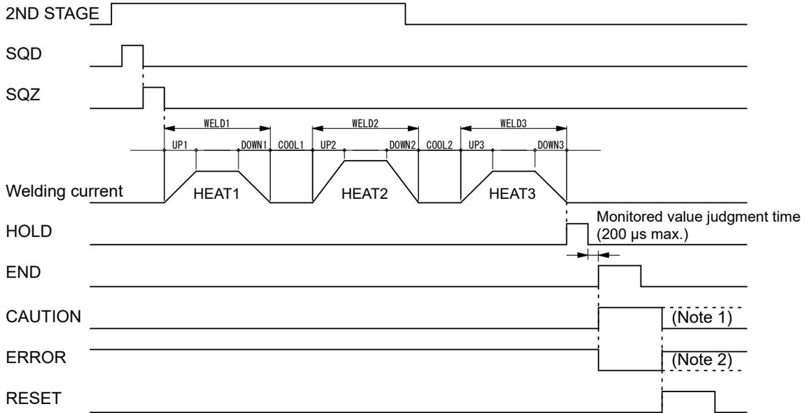
(Note 1) The CAUTION output is ON until the RESET signal or the next 2ND STAGE signal is input.
