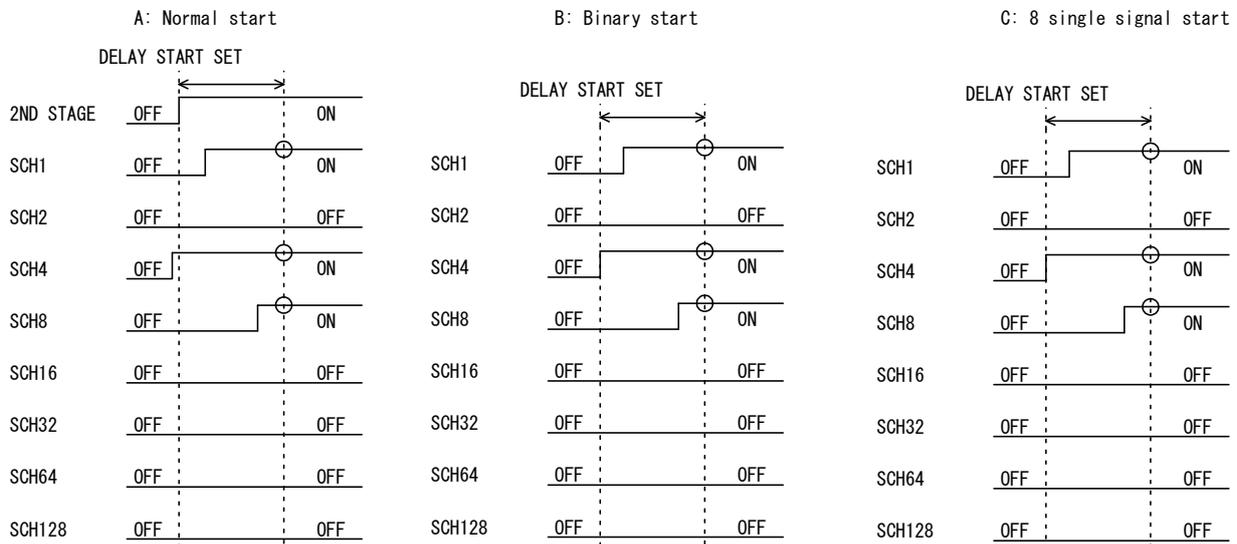
In 4) and 5), up to 255 schedules can be used by combining schedule signals SCH1/2/4/8/16/32/64/128 in binary. In Fig. B: Binary start, schedule No. 13 is selected since signals SCH1/4/8 are determined.
