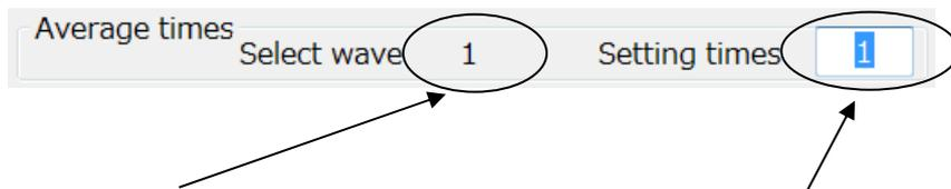
The number of moving average of the waveform when obtaining data selected in the waveform data list on the Basis Waveform Calculation Window is displayed. When waveforms that have different number of moving averages are selected, nothing is displayed.
