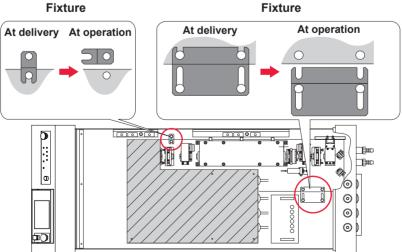
⇒ For moving the laser welder after it is installed, fix the laser oscillator with the fixture to put it to the same status as when it is delivered.
