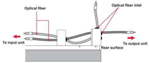
There are 2 optical fiber inlets, namely, one on the top surface and the other on rear surface of the main unit.
