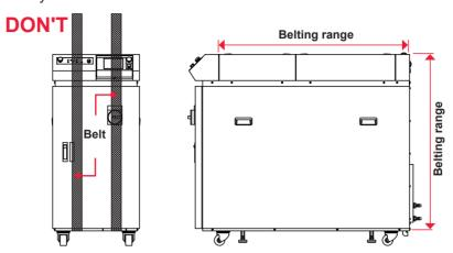
⇒ Put the laser welder in close contact with the two surfaces of floor and wall and fix it securely with a belt. Be sure to use cushion between the Laser and belt not to hurt the Laser.
