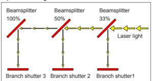
Laser light is reflected on the beamsplitter and split, and then simultaneously transferred from opened branch shutters 1, 2, and 3.
