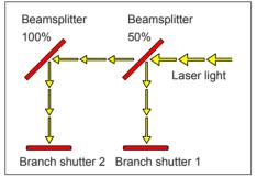
Laser light is reflected on the beamsplitter and split, and then simultaneously transferred from opened branch shutters 1 and 2.
