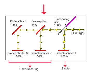
In the case of 2-powersharing delivery + single delivery, laser light is output from branch shutters 1 and 2 as 2-powersharing delivery and from branch shutter 3 as single delivery, depending on a difference in beamsplitter mounting condition.
