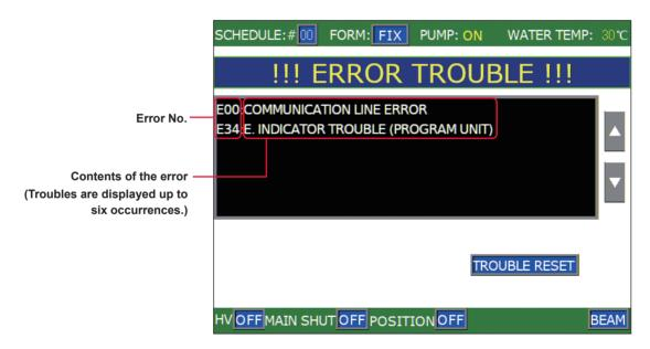
High voltage "-": State of high voltage doesn't change even if an error/fault occurs. High voltage "OFF": High voltage is turned off automatically if an error/fault occurs. Error/Fault signal "-": Error/Fault signal is not output if an error/fault occurs.
