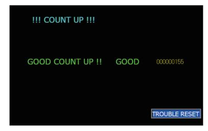
Press the "TROUBLE RESET" button to return the current screen to the initial screen.
