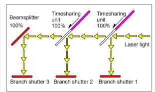
Laser light is reflected on the beamsplitter by operated timesharing unit and transferred from opened branch shutter 3.
