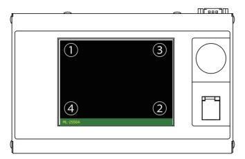
(2) While the model name screen is displayed (for about 3 seconds), press the corners of the touch panel display in the order shown in the figure above. The INITIALIZE screen appears.
