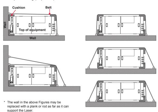
⇒ When it is expected that the Laser may bounce during transportation, belt the Laser longitudinally.
