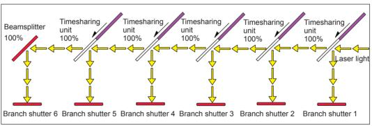
Laser light is reflected on the beamsplitter by operated timesharing unit and transferred from opened branch shutter 1 to 6.
