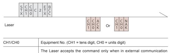
control (RS-485 CONTROL) mode. It returns a [NAK] when in any other
