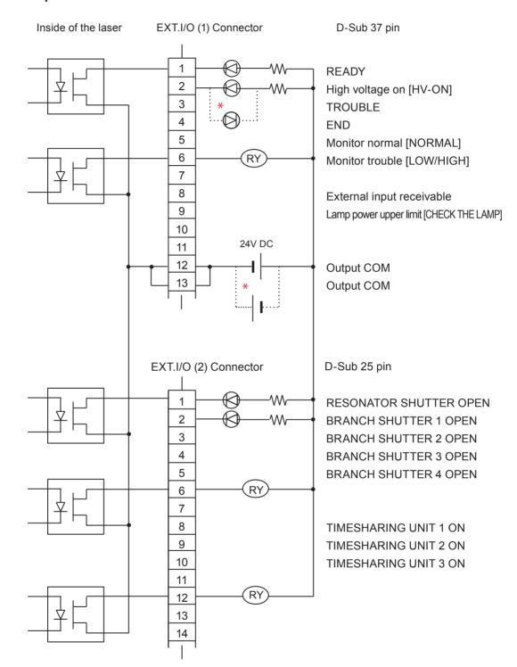
Type of output: Photo MOS relay output Rating of output: 24 V DC, 20 mA max.
