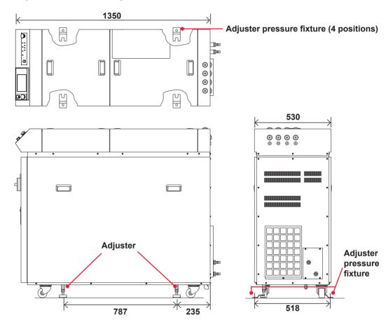
(2) Fix each adjuster on the floor by using a connecting apparatus such as anchor.
