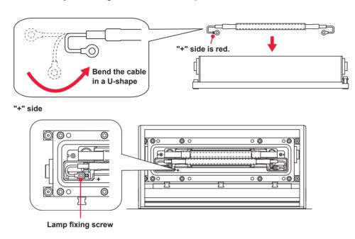
(3) Tighten the bolts on both ends of the flashlamp to fix the flashlamp.
