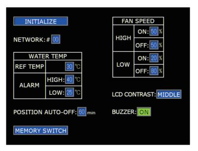
Unless the CONTROL keyswitch is OFF, the INITIALIZE screen does not appear.
