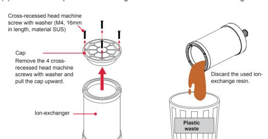
(4) Remove the cap of the ion-exchanger and discard the used ion-exchange resin.
