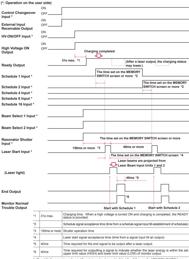
In \*2 and \*4, the acceptance time is 16 ms but can be changed to 0.1, 4.0 or 8.0 ms on the MEMORY SWITCH screen.
