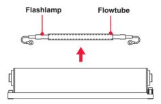
⇒ When removing the flashlamp, you can see the net in the laser chamber. Check this mesh portion and remove dust or glass fragments with tweezers if any.
