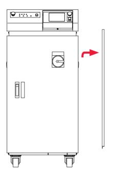
Remove the screws of the side cover, raise the cover, and pull it out forward.
