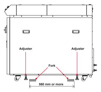
Figures below show example forking; insert the forks fully till the points appear from under the Laser.
