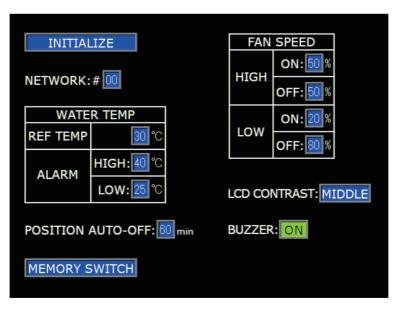
Unless the CONTROL keyswitch is OFF, the INITIALIZE screen is not displayed.
