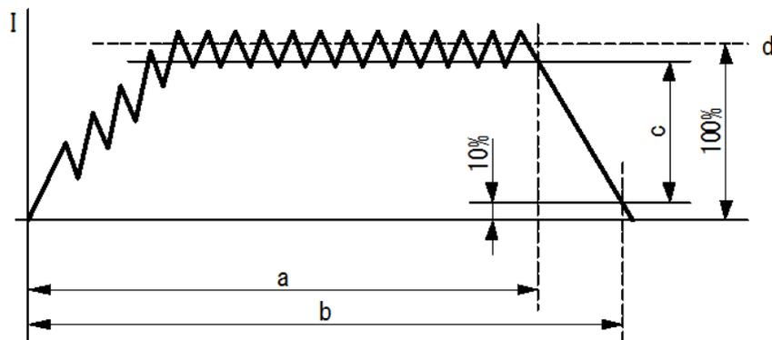
a: Weld time till the fall level b: Flow time c: Fall level 10 to 90% d: Current effective value
