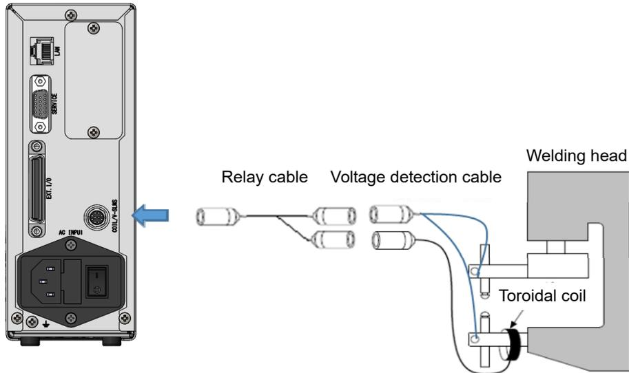
When connecting the voltage detection cable, be careful with the following:
