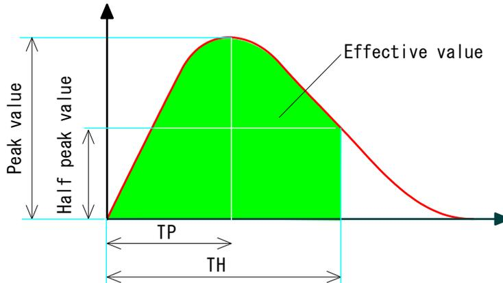
In the current measurement mode CAP-S or CAP-L, the effective value over the TH is displayed.
