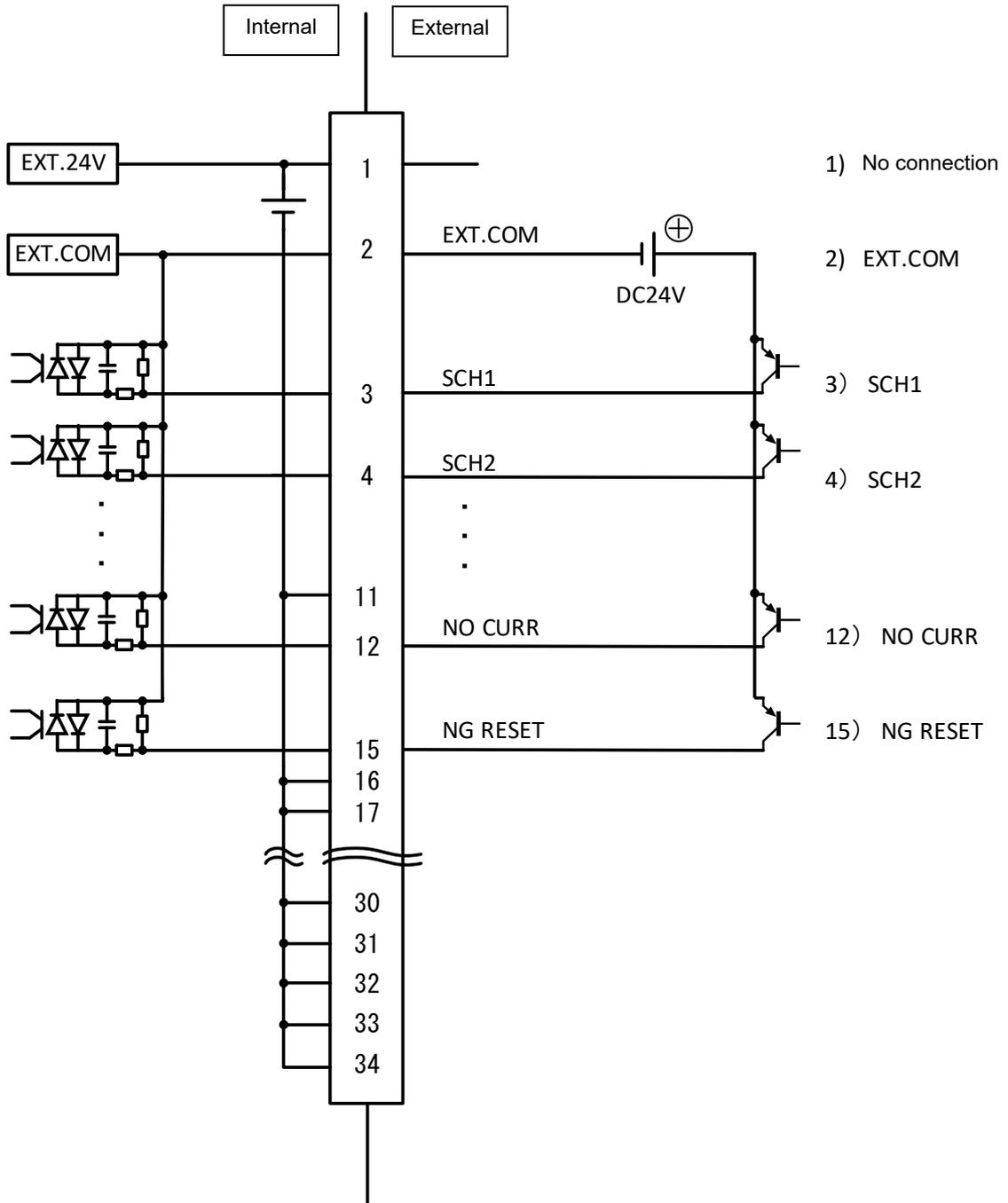
d. Connection with Device Featuring NPN Open Collector Output (when Using External Power Supply)
