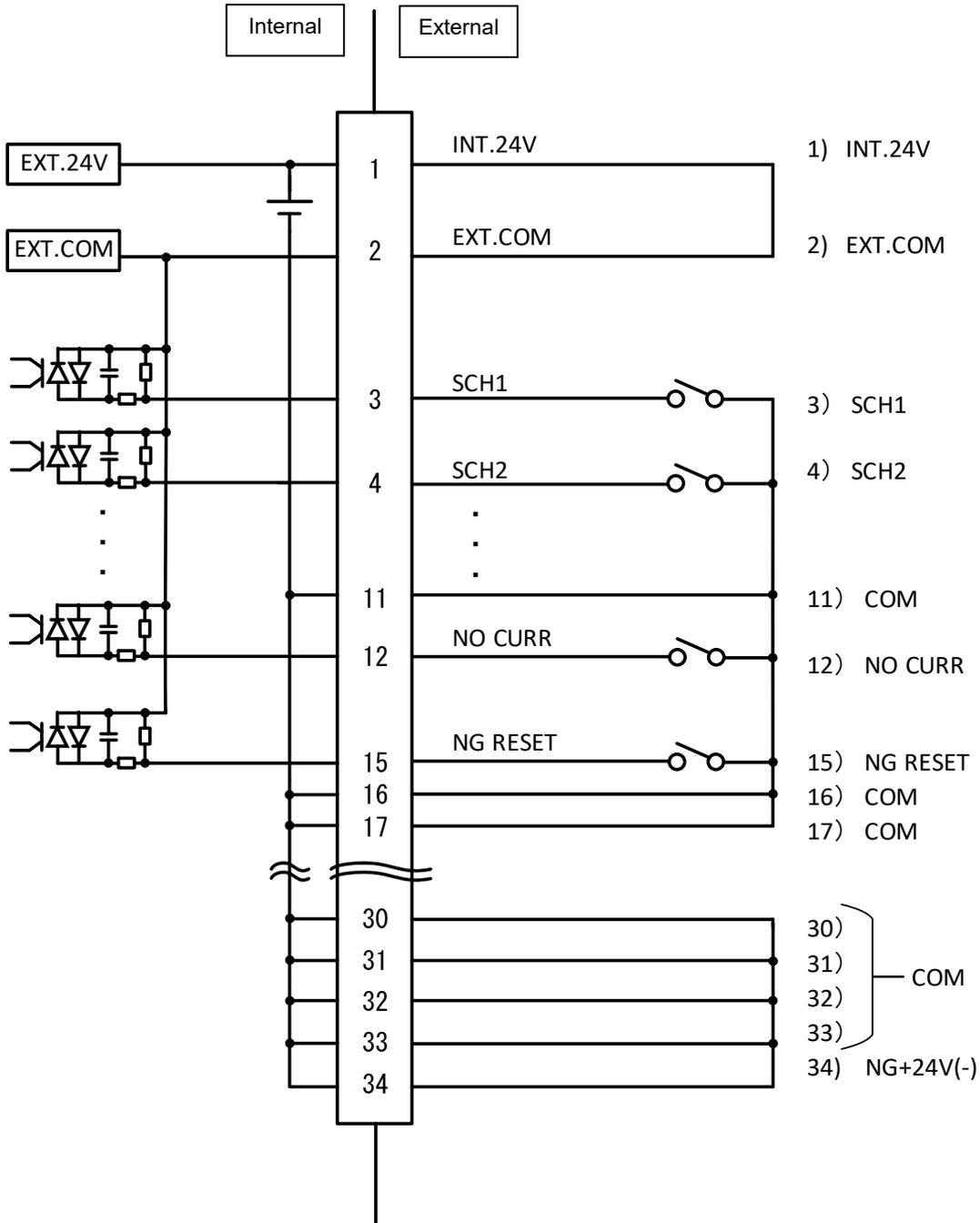
b. Connection with Device Featuring NPN Open Collector Output (when Using Internal Power Supply)
