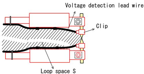
When the voltage detection cable wires are placed as shown to the left, voltage induced by the welding current is added to the voltage between tips. When monitoring voltage, fasten the lead wires so that the loop space S does not change and induction voltage does not fluctuate.
