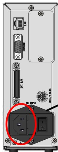
Do not connect the power cable to the power supply connector when using 24 V DC.
