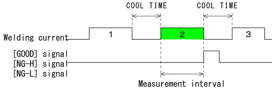
If the welding current doesn't reach the stage set in the impulse measurement, the [NG+24V] signal and the [NG-H] signal are output. For details, see [5. (2) Description of the External I/O Signals].
