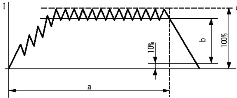
a: Weld time till the fall level b: Fall level 10 to 90% c: Current peak value
