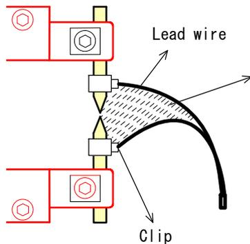
Make the distance between clips as small as possible, and twist the lead wires together so that induction voltage is reduced and the voltage between tips can be measured accurately.
