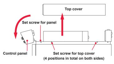
(3) Loosen the screws to clear the fixture, so that the laser oscillator is put in a remote place from the oscillator base.
