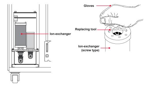
(4) Remove the cap of the ion-exchanger and discard the used ion-exchange resin.
