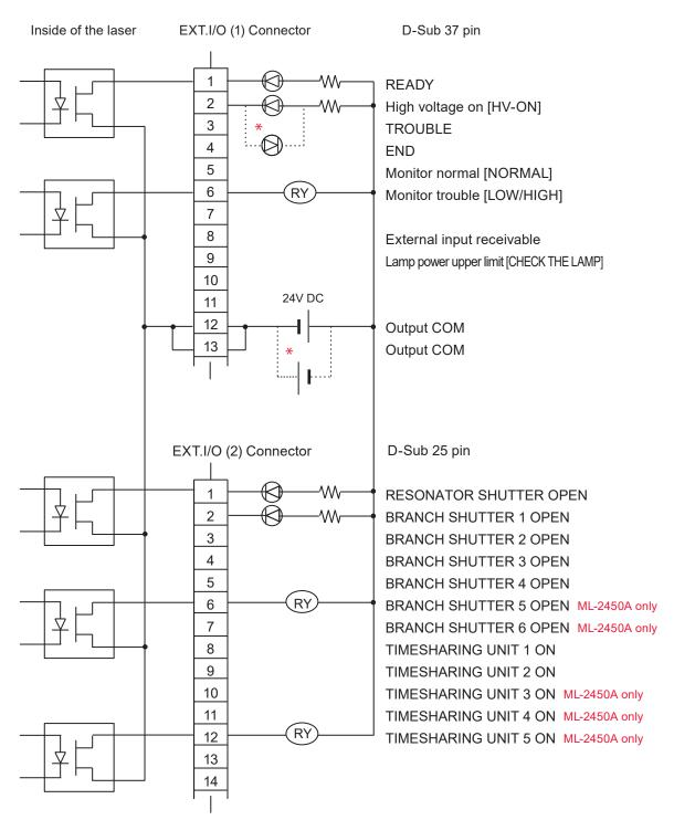
Type of output: Photo MOS relay output Rating of output: 24 V DC, 20 mA max.
