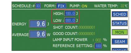
When laser light is out of the set allowable energy range, a monitor error is output.
