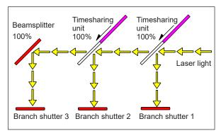
Laser light is reflected on the beamsplitter by operated timesharing unit and transferred from opened branch shutter 2.
