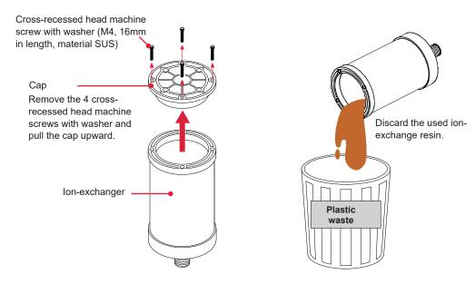
⇒ Dispose of the used ion-exchange resin together as plastic waste.
