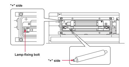
⇒ When returning the flashlamp into the laser chamber, set the lamp-side fixture correctly in the chamber-side fixture.
