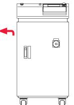
Remove the screws of the side cover, raise the cover, and then pull it out forward.
