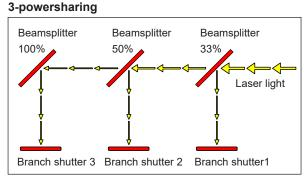
Laser light is reflected on the beamsplitter and split, and then simultaneously transferred from opened branch shutters 1 and 2.
