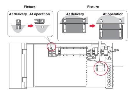
⇒ For moving the laser welder after it is installed, fix the laser oscillator with the fixture to put it to the same status as when it is delivered.
