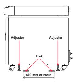
Figures below show example forking; insert the forks fully till the points appear from under the Laser.
