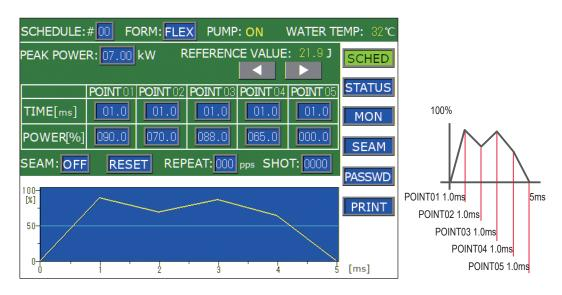
⇒ At the leading edge of waveform, an overshoot (higher form than the set value) may occur. In this case, extend "POINT 01" by 0.1 to 1.0 ms.
