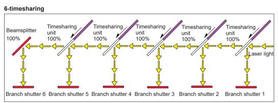
Laser light is reflected on the beamsplitter by operated timesharing unit and transferred from opened branch shutter 1 to 6.
