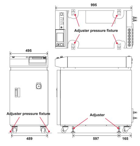
(2) Fix each adjuster on the floor by using a connecting apparatus such as anchor.
