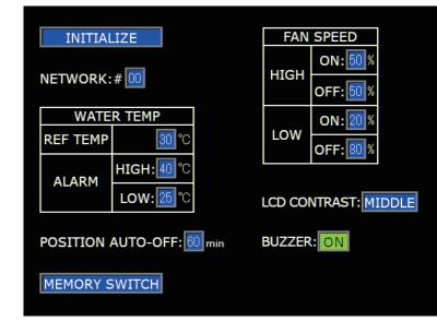
⇒ Unless the CONTROL keyswitch is OFF, the INITIALIZE screen is not displayed.
