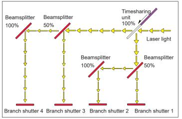
Laser light is reflected and branched on the front or rear beamsplitter by the operation of the timesharing unit. The beams are simultaneously transmitted when branch shutters 1 and 2 or 3 and 4 are opened.
