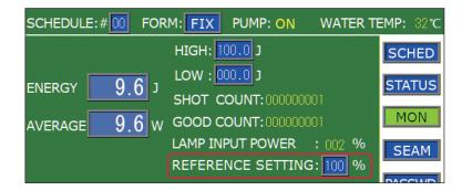
⇒ If the laser welder is used in the status where 80% or more is displayed in "LAMP INPUT POWER", the flashlamp replacement cycle may be shortened.
