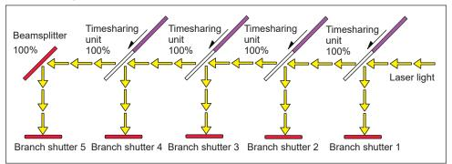
Laser light is reflected on the beamsplitter by operated timesharing unit and transferred from opened branch shutter 1 to 5.
