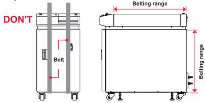
⇒ Put the laser welder in close contact with the two surfaces of floor and wall and fix it securely with a belt. Be sure to use cushion between the Laser and belt not to hurt the Laser.
