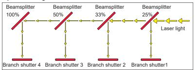
Laser light is reflected on the beamsplitter and split, and then simultaneously transferred from opened branch shutters 1, 2, 3, and 4.
