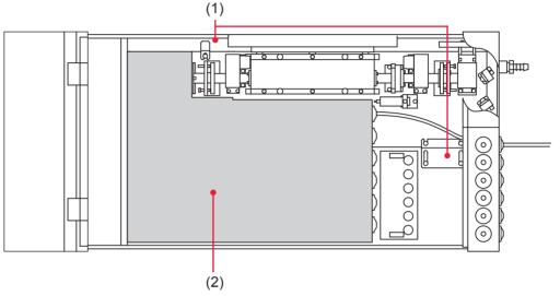
Status where the branch unit cover is removed (for 3-powersharing/2-timesharing delivery specification)
