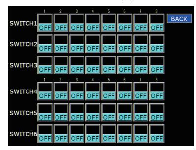
(2) Press the setting buttons of "1" to "6" of "SWITCH 4" to set the branch shutter No. to be operated to ON.
