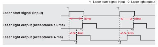
⇒ The laser start signal acceptance time and the schedule signal acceptance time are common. A different value cannot be set for the respective time.
