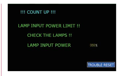
When this screen appears, output pin No.9 (upper limit of lamp input) of the external output signal EXT.I/O (1) connector is open-circuited for output.
