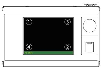
(2) While the model name screen is displayed (for about 3 seconds), press the corners of the touch panel display in the order shown in the figure above. The INITIALIZE screen appears.
