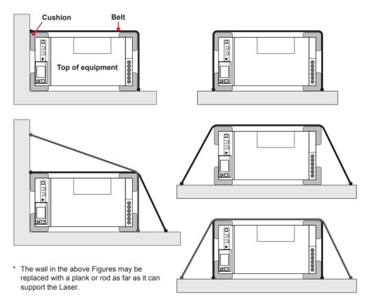
⇒ When it is expected that the Laser may bounce during transportation, belt the Laser longitudinally.
