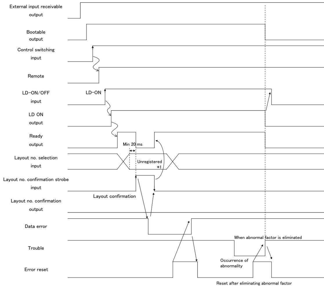
\*1 When an unregistered number is selected at the time of the layout no. confirmation strobe input, the layout no. before confirmation is selected.
