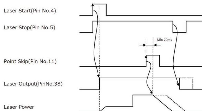
\*The laser operates as above, but the layout operates only for the time set in advance in the layout of SWDraw3. (In the figure above, laser output signal)
