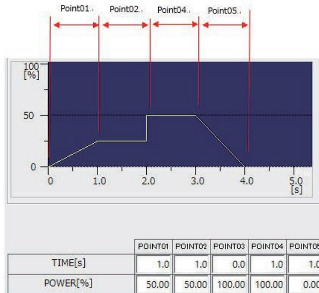
(Example) When point skip is executed in the middle of point 04 with the above waveform settings.
