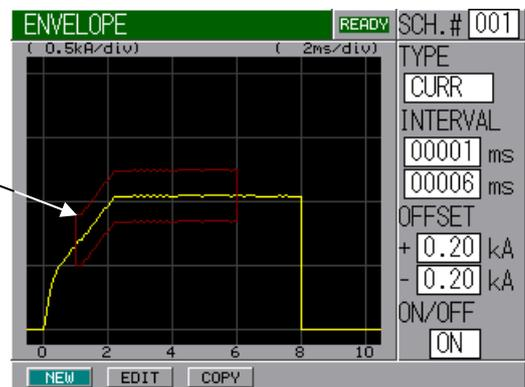
When displaying the monitored screen, Envelope Waveform will appear.
