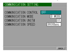
To perform communication, set items referring to 6. (6) **@COMMUNICATION CONTROL** to **@COMMUNICATION SPEED**.
