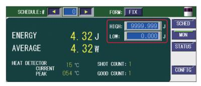
⇒ When laser light is out of the set allowable energy range, error No.035/LASER POWER OUT OF RANGE occurs and a monitor trouble is output. (Pin No.20 of the EXT. I/O (1) connector is closed for the time set on the CONFIG screen after a laser output.) When the total laser output time is 0.5 s or less in the CW mode, however, a monitor trouble does not occur even if laser light is out of the range.
