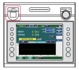
(6) Press the "LD" setting button to set it to OFF and press the "END" button.
