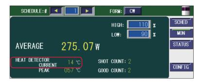
When the indicated temperature is low, check that the protective glass of the output unit is not dirty. Note that the low temperature is also displayed in an environment where there is much dust or gas, and humidity is high. On the contrary, when the high temperature is displayed, check that there is no high-temperature heat source or lighting nearby. If there are no problems in particular, adjust the correction factor to use it.
