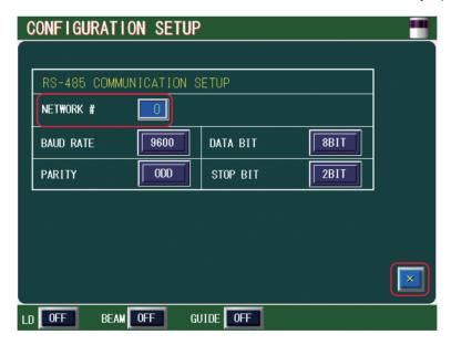
(2) Press the "X" button. Returns to the CONFIG screen.
