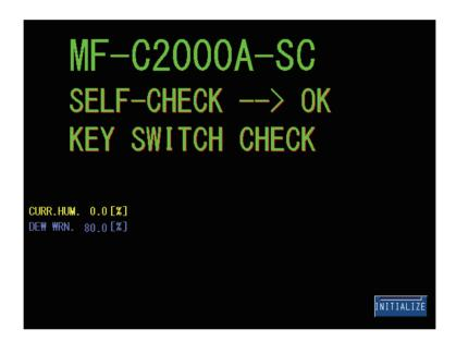
(4) Turn ON the CONTROL keyswitch. The engine (oscillator) is automatically checked.
