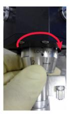
(3) Pull out the connector section about 2 mm and turn it in the direction of the arrow 2.
