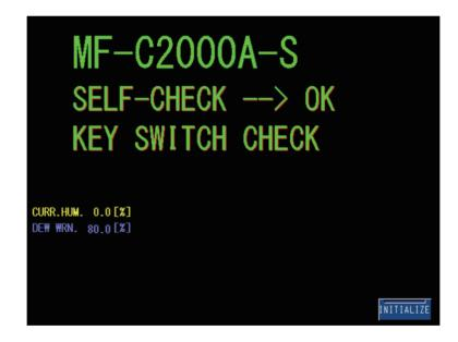
When the dry air unit (option) is equipped, the "CHILLER" button is displayed on the KEY SWITCH CHECK screen. The chiller is normally kept running, but if you want to stop it, press the button twice within a second to switch between stop and
