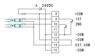
• When PNP transistor (source type) on PLC is used as input terminal of I/O connector
