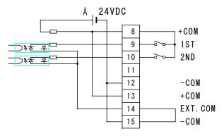
· When NPN transistor (sink type) on PLC is used as input terminal of I/O connector
