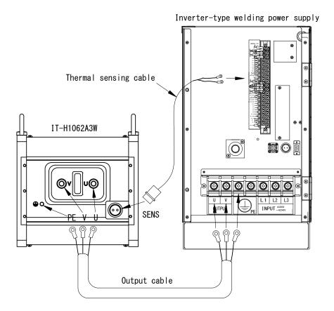
The output cable and thermal sensing cable are sold separately. The terminal screw of **IT-H1062A3W** is M8 (PE terminal is M6).
