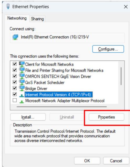
8) Input the IP address. As in the following figure, set any value other than [192.168.1.40] for IP address, and set [255.255.255.0] for Subnet mask, and then click the [OK] button.
