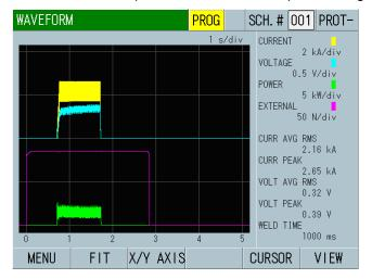
Displays ON (+0 V) to 500 N (+10 V) with a load cell amplifier prepared separately.
