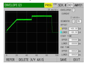
9) Touching the REFER key and selecting YES displays reference waveform and envelope setting. You can also check the detailed data of time axis and vertical axis by touching the X/Y AXIS key. After check, touch the BACK key and return till the REFER key is shown.
