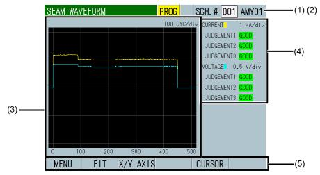
Waveform of intermittent seam current / voltage
