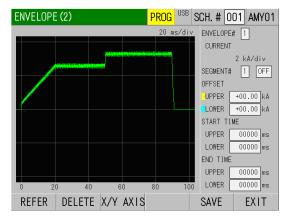
8) Select 1 for ENVELOPE#, select 1 for SEGMENT#, and change OFF to ON. Set upper and lower limit values in UPPER and LOWER of OFFSET. As the time range to judge the upper and lower limit, set from START TIME to END TIME. The time range can be set for UPPER and LOWER respectively.
