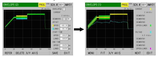
12) Touch the EDIT key again, select 3 for SEGMENT#, and change OFF to ON. Perform steps 6) to 10). Be sure to perform from REFERENCE to SAVE for each setting of SEGMENT.
