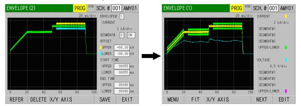
13) Similarly, select 2 for ENVELOPE# for WAVEFORM 2 and perform settings of SEGMENT#1 to 3. Be sure to perform from REFERENCE to SAVE for each setting of SEGMENT.
